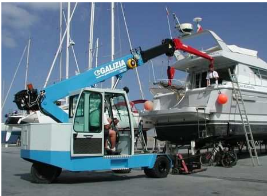
The 8 tonne G8 fitted with fly jib and hoist
