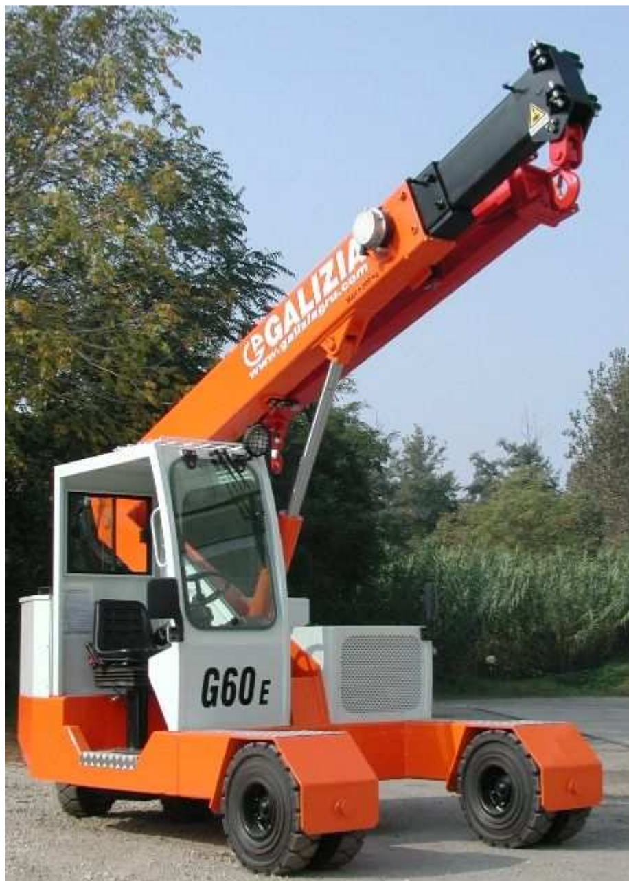
The 6 tonne Galizia G60E with battery power
